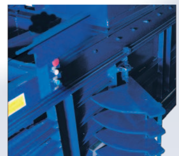
Elephant Ear Dawg Assembly Used On Horizontal Foam Balers is a Max-Pak Innovation That Provides Maximum Holding Capacity for Baling Foam.
